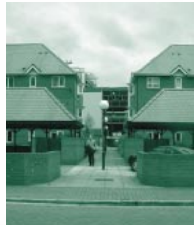
An example of good footpath design which is short, direct, well lit and open to surveillance.
